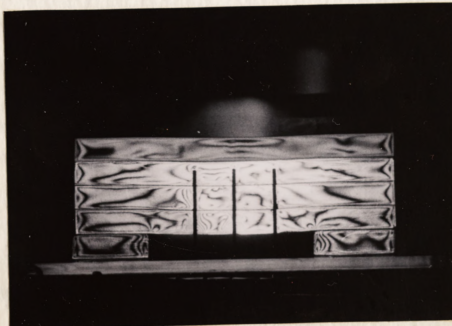
Picture 22. Test (8): Fringe Pattern of an Unsymmetrical Model with three Vertical Roof Bolts.
