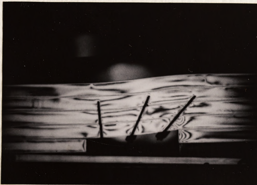
Picture 24. Test (15): Fringe Pattern of an Unsymmetrical Model with three Roof Bolts ( 90^\circ , 60^\circ and 45^\circ ).
