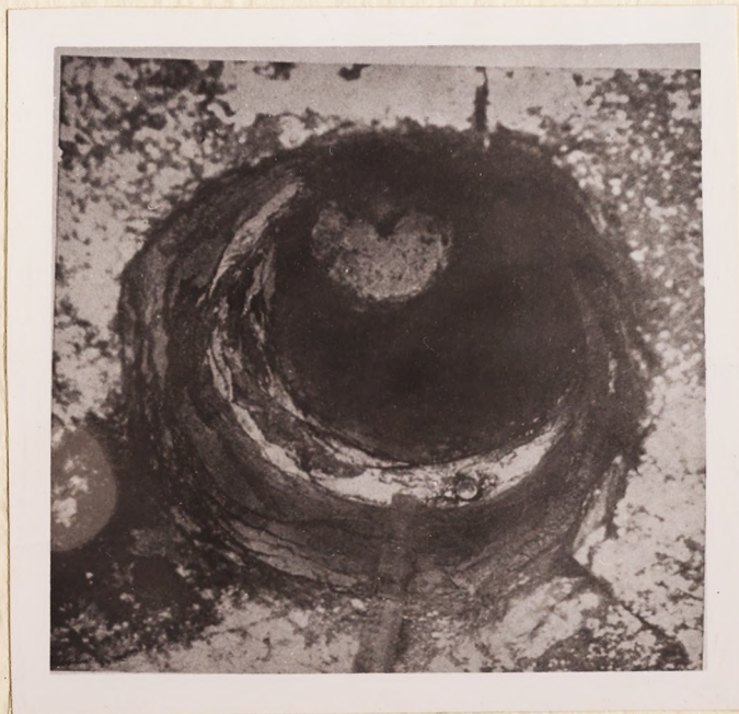
Picture 7. "Quarter-Moon" Shape in a Borehole caused by Bed Displacement.
