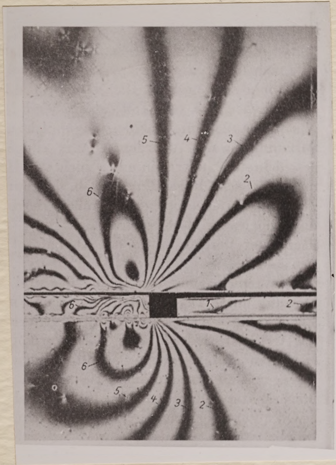
Picture 3. Stress Distribution in the Surroundings of a Long Wall Operation with thick Beds (after Sonntag)
