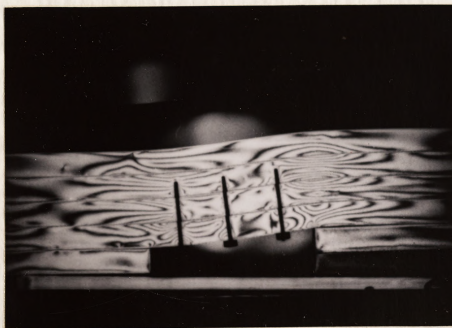
Picture 28. Test (19): Fringe Pattern of an Unsymmetrical Model with three vertical Roof Bolts.
