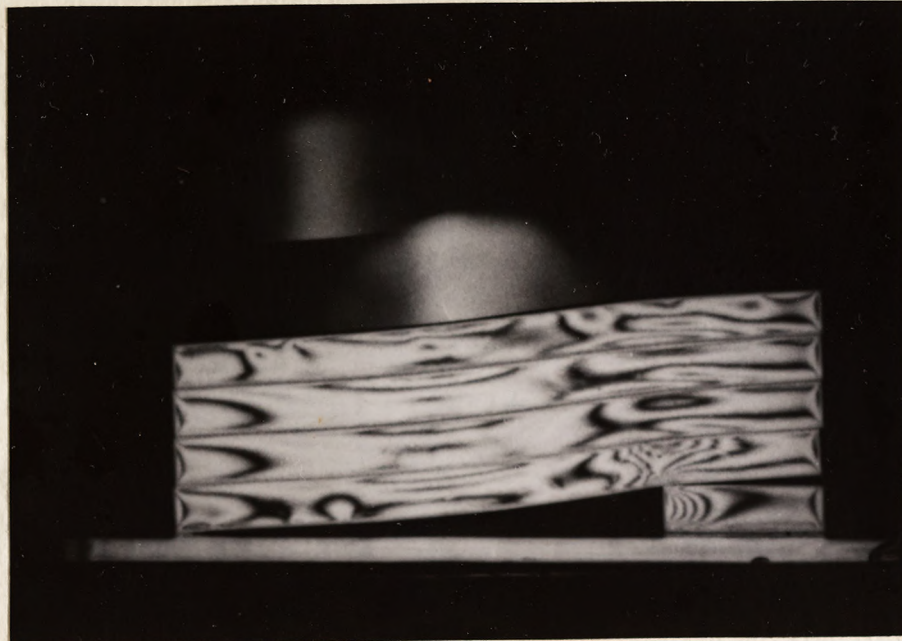
Picture 21. Test (13): Fringe Pattern of an Unsymmetrical Model.
