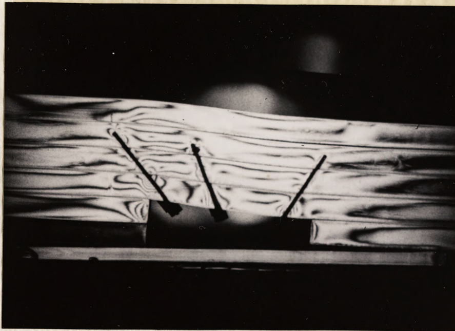
Picture 29. Test (20): Fringe Pattern of an Unsymmetrical Model with three Roof Bolts ( 45^\circ , 60^\circ and 60^\circ ).
