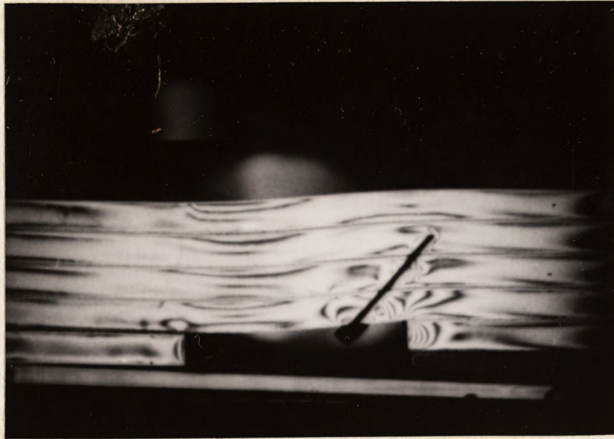
Picture 25. Test (16): Fringe Pattern of an Unsymmetrical Model with one Roof Bolt ( 45^{\circ} ).
