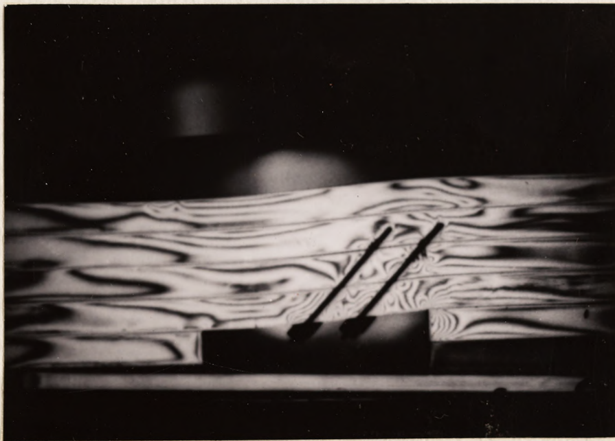
Picture 26. Test (17): Fringe Pattern of an Unsymmetrical Model with two Roof Bolts ( 45^{\circ} and 45^{\circ} ).
